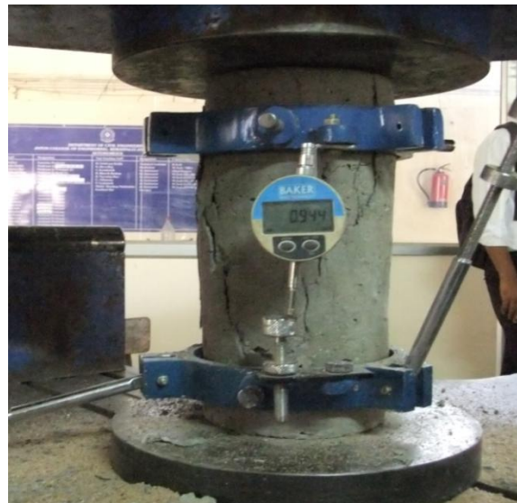
Fig. 5 Cylindrical specimen subjected to axial compression
